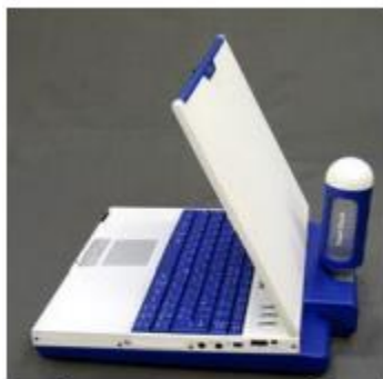
A laptop powered by a direct methanol fuel cell
